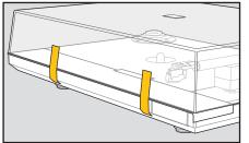
Insert dustcover hinges fully, then use tape to secure the dustcover to the body of the turntable so it cannot open.
