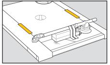
Attach two foam strips across the front and back of turntable.
