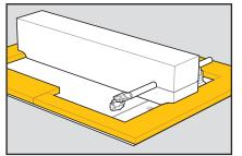
Place periphery foam strip across the top of the turntable plinth. This should have a snug fit against the foam block supporting the tonearm.
