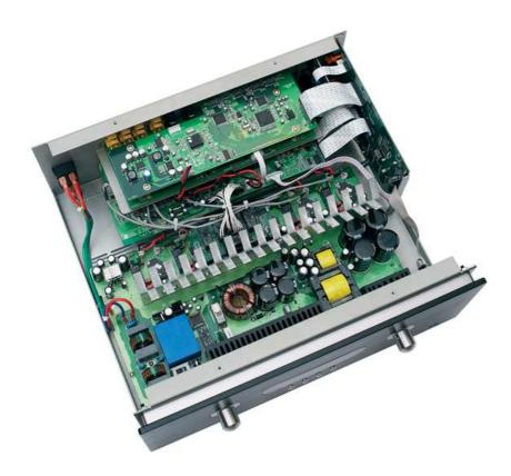
Primare's UFPD (Ultra Fast Power Device) provides for the possibilities of an 'audiophile' Class D design. It is a Class D technology which has a consistent 26dB feedback loop gain across the entire audio range and is stable way beyond the audio band. This is quite easy to achieve in conventional linear 'continuous signal' amplifiers, but much more difficult in 'non-continuous' high speed switching amplifiers.
