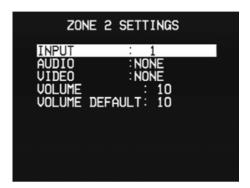
For each input the **ZONE 2 SETTINGS** menu allows you to specify an analogue audio input and an S-Video or composite video input to be output to the Zone 2 outputs.
