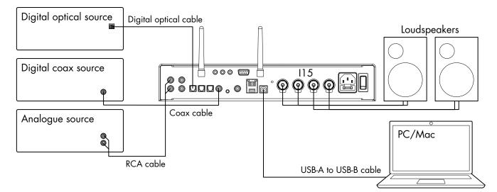
These methods of playing music from the 115 involve connecting the source to the 115 via a cable, and don't require Wi-Fi, Ethernet, or Bluetooth.
