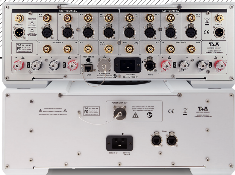
ABOVE: Six line ins, four on balanced XLRs, are offered alongside a recorder loop. Balanced and single-ended (RCA) pre-outs are included together with dual speaker terminals for bi-wiring. Auxiliary power amp PSU connects via a thick umbilical
