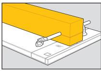
Secure tonearm with supplied foam stabilizer block. Then wrap unit with supplied plastic bag.
