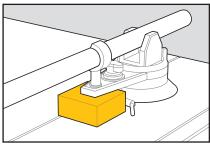
Place small foam block underneath the tonearm platform for support.
