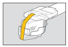
Install the cartridge stylus guard and use a small piece of masking tape to hold it in place.
