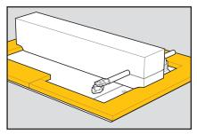
Place periphery foam strip across the top of the turntable plinth. This should have a snug fit against the foam block supporting the tonearm.
